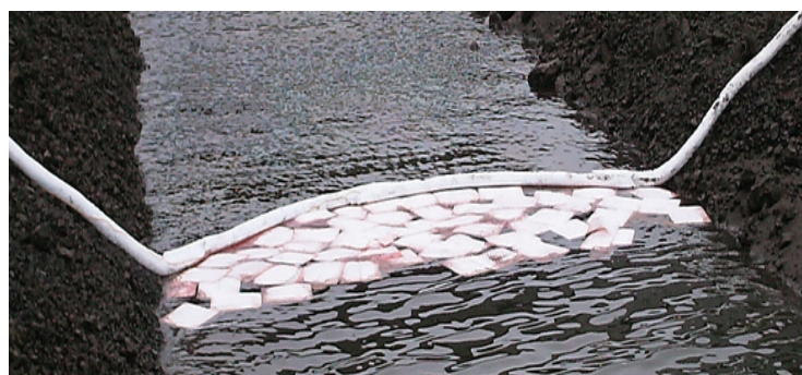
Figure 2. Application of the absorbent as a hydrocarbon filter 19
