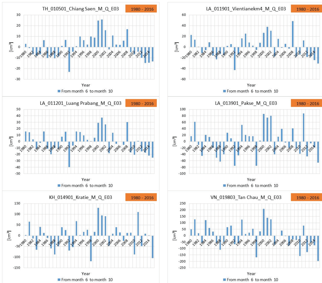
Figure 15: Gain and loss of flow volume against long-term averages at selected stations since 1980 (June-October)
